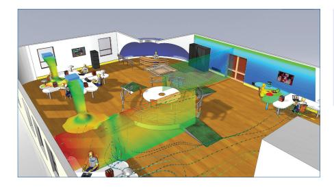
Mentor Graphics' Mechanical Analysis Division has been a leader in the simulation of airflow and temperature for the built environment since 1989. With FloEFD's concurrent CFD, software that connects directly with your CAD software, users can simulate airflow and heat transfer using 3D CAD models directly, with no need for data translations or copies.
